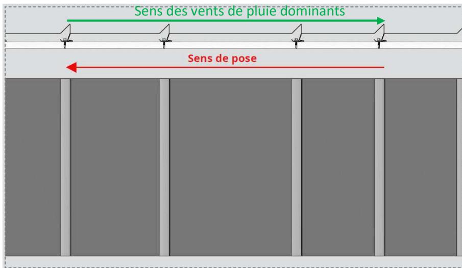
**Figure 18 – Sens de pose vertical**
